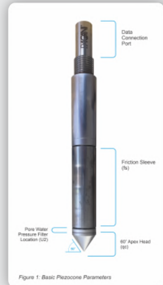
Figure 1: Basic Piezococone Parameters
