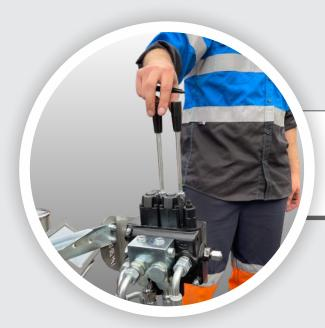
Onboard CPTu controls for precision testing.
