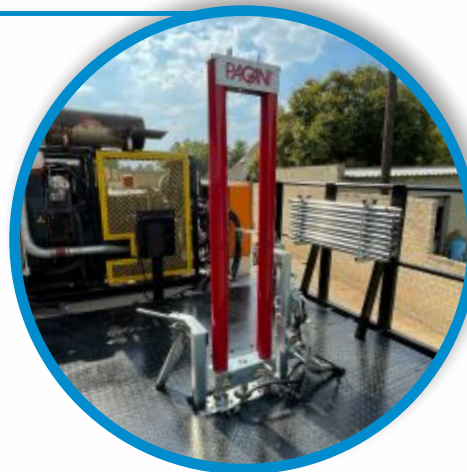
Pagani CPT Mast 150 mounted on a Morooka track-based rig. (closed position)
