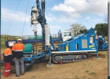
Sonic drilling can be employed in virtually any application where good core recovery is a requirement in softer ground.
