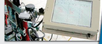
The TGAS08 is equipped with a GPS location module to obtain positioning information and a GPRS module for sending test results directly to a computer located anywhere via a simple email. If there is no GSM network coverage, data can be downloaded directly on to a standard USB stick.
