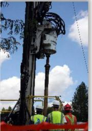
The Sonic 450-24 rig is able to provide continuous core samples to depths of more than 100 meters without using any drilling mud. As a result, sonic drilling can be employed in many applications including geotechnical and geothermal projects, environmental investigations and mineral exploration.
